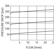
The Performance Chart illustrates flow handling capacity at max. setting for each spring range option. Pressure rise will vary with spring (range) and with setting within range due to flow forces.
